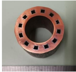
Figure 10: Cross-section of sample A viewed from the horizontal direction. Reprinted from [23] .
