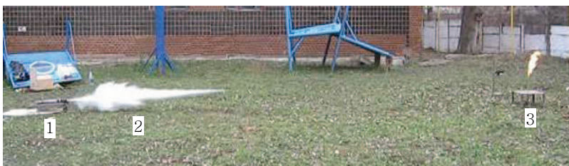
Figure 7: The middle stage of impulse liquid jet propagation. 1 – powder impulse water-gun, 2 – impulse jet, 3 – gas blow-out
