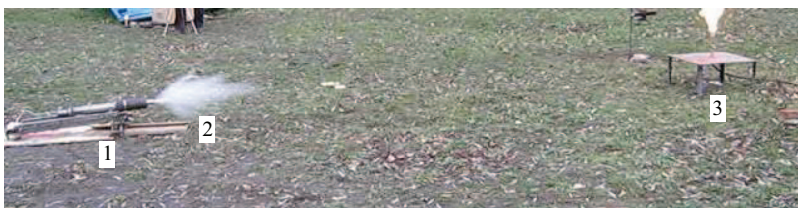
Figure 6: The initial stage of liquid jet formation from impulse water-gun. 1 – powder impulse water-gun, 2 – impulse jet, 3 – gas blow-out
