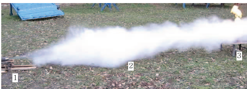
Figure 8: The last stage of putting out of gas blow-out. 1 – powder impulse water-gun, 2 – impulse jet, 3 – gas blow-out
