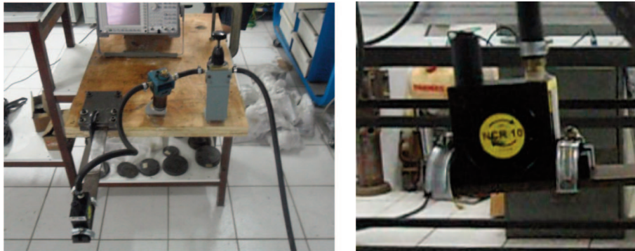
Figure 5: a) Experimental setup for conducting treatment by vibration; b) Detail of the pneumatic vibrator
