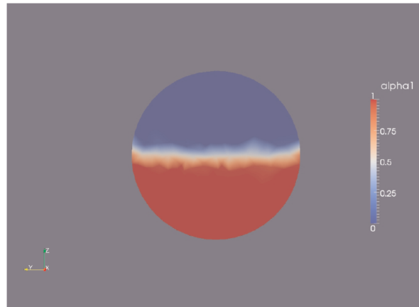
Figure 14: Volume fraction of the water in a pipe cross section (stratified flow)
