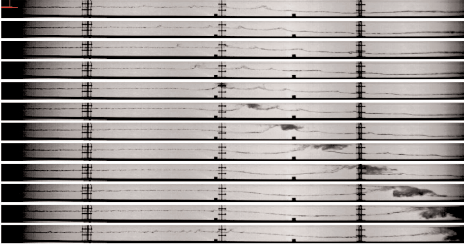
Figure 12: Picture sequence of the quasi-periodic slug flow with a \Delta t of 50 ms between two consecutive photos; depicted part of the channel is up to 3.2 m downstream of the inlet [37]
