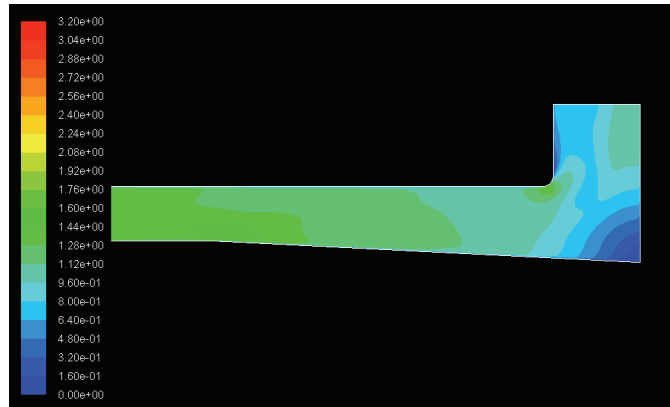
Figure 8. Velocity field for modified chamber with a trench 2 meter deep and output section expanded to double and curvature radius of 1 meter
