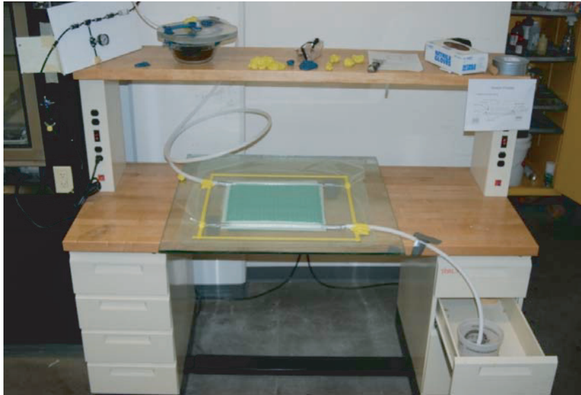
Figure 2. Fabrication of samples using the VARTM process.
