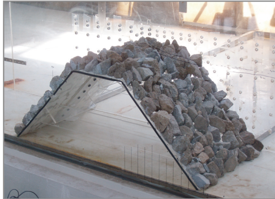
Figure 2 Rough impermeable model.
