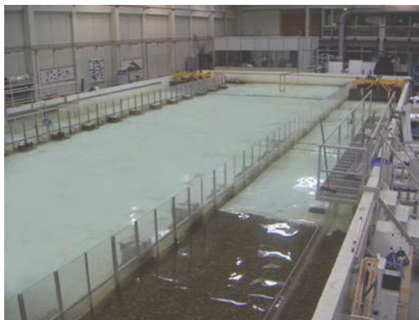
Figure 1 Wave tank ( 28 \times 12 \times 1 \text{ m}^3 ) of the Hydraulics Laboratory of FEUP.
