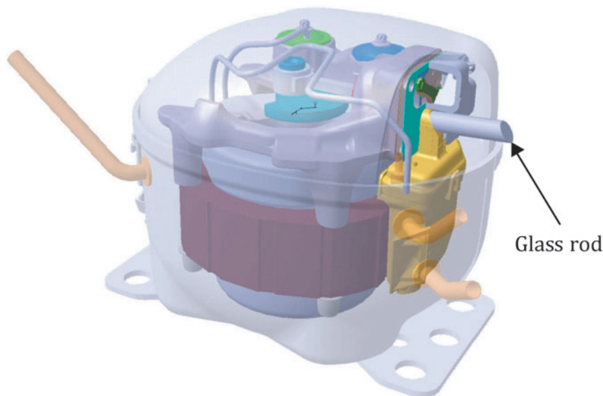
Figure 12 Measuring setup for the valve measurements.
