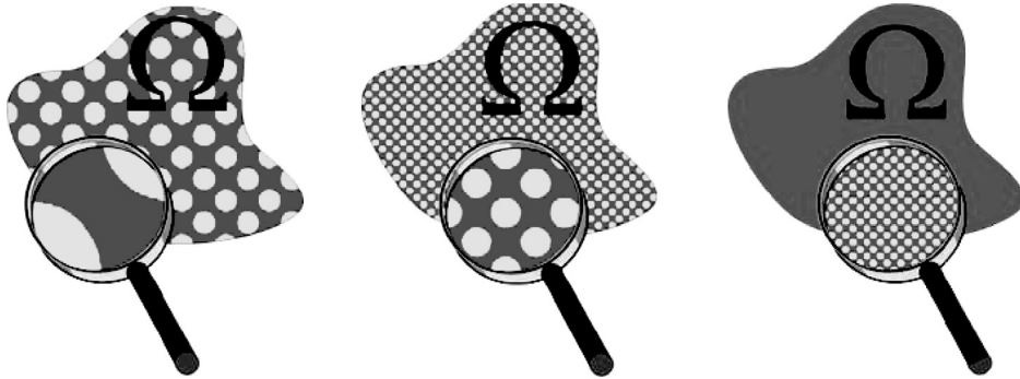
Figure 8 The microstructure becomes finer as the parameter \varepsilon becomes smaller (left to right).
