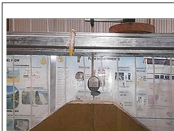
Figure 6. The digital dial gauge is used to measure settlement.
