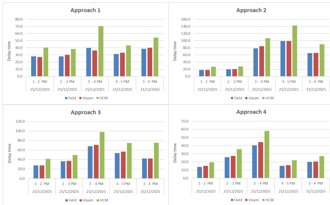
Figure 8: Delay Time Comparison at El-Safera Aziza Signalized Roundabout
