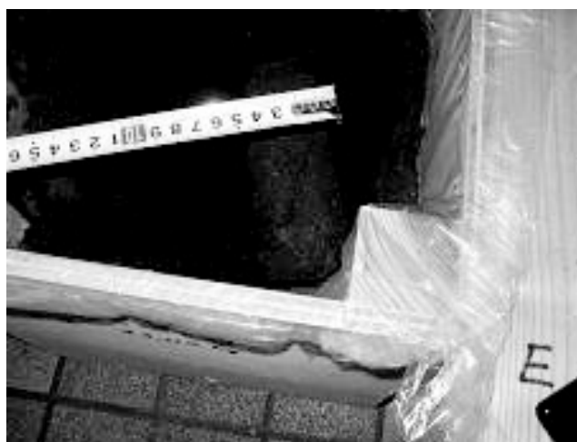
Figure 10 Photograph of the remaining frozen layer 3 hours after shock loading in the case of Lot. E.
