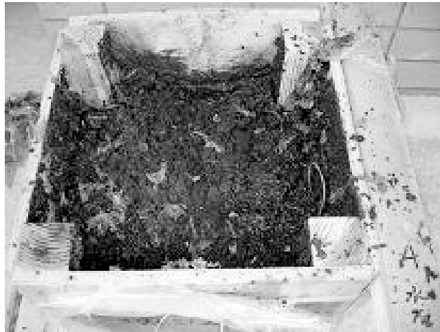
Figure 7 Photograph of the frozen soil box immediately after shock loading in the case of Lot. A.
