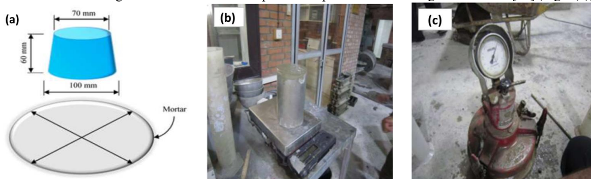
Fig. 7. (a): Mini-slump test, (b): Fresh density test, (c): Air content percentage test.
