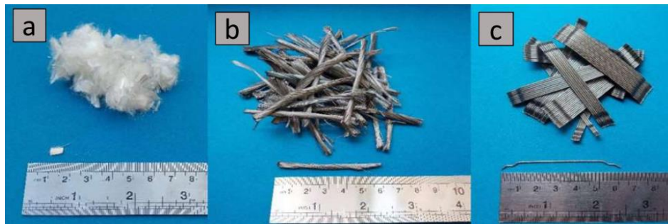
Fig. 4. The shape of fibers. (a) PVA Fiber; (b) Synthetic fiber; (c) Hooked steel Fiber.
