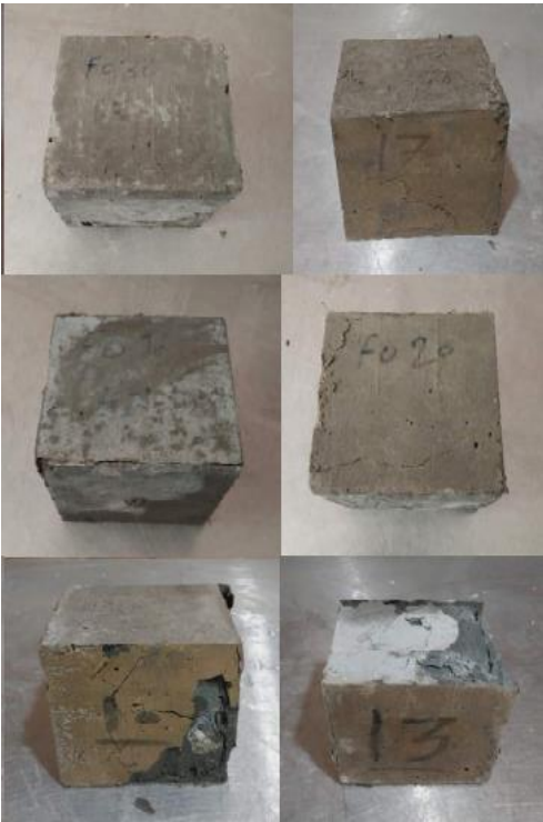
Fig. 12. Compression samples tested.
