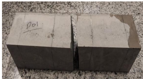
Fig. 15. Flexural beam specimen tested; S0F0P0.
