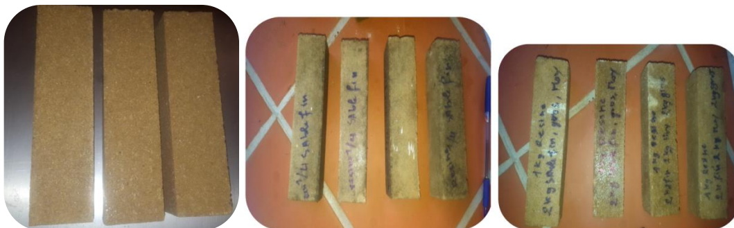
Figure 5. Epoxy resin mortar with silica sand ( a: fine sand, middle sand, coarse sand)
