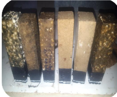
Figure 8. Water absorption by capillary test
