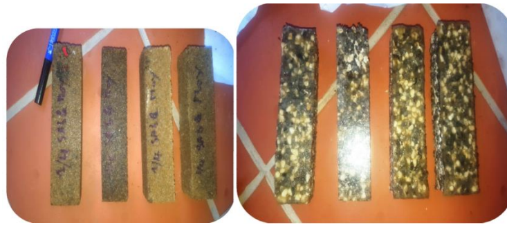
Figure 6. Epoxy resin mortar with marble aggregate (Marble sand)
