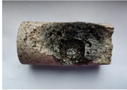
Fig. 5 Rock sample melting under microwave irradiation at 5 kW for 5 min
