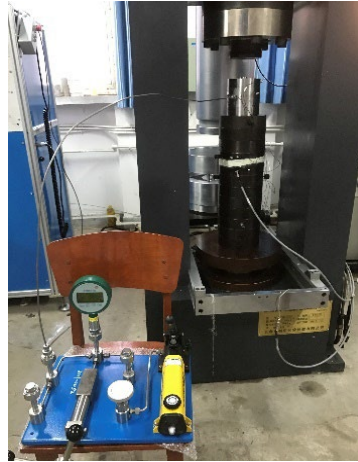
(b) TAW-2000 electro-hydraulic triaxial testing machine
