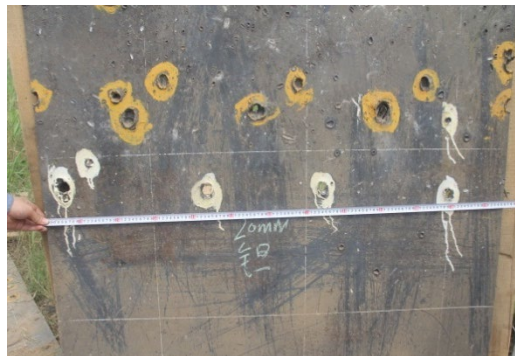
(a) Perforation of 20 mm target plate
