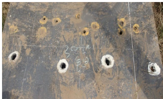
(b) Perforation of 30 mm target plate
