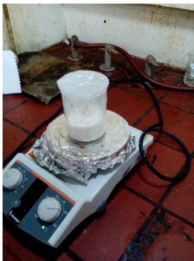
Figure 3: Initial cell prepared on a magnetic stirrer
