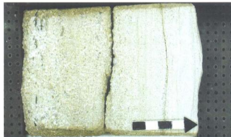
Depth: 3320.35-3320.48 m Lithotype: 2A Facies: Tidal channel-fill facies
