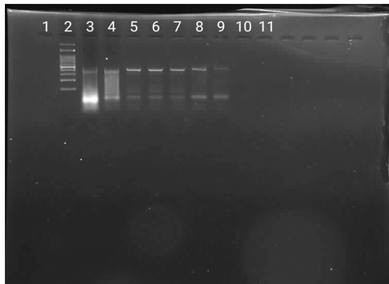
Figure 7: Determining the sensitivity of the optimized PCR test using different DNA dilutions from standard Haemophilus influenzae . Column (2): DNA 100 bp ladder, columns 3 to 11 are related to different dilutions of Haemophilus influenzae DNA. Column 2: Negative control
