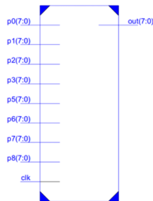
Fig. 7 Schematic of Sobel edge detection
