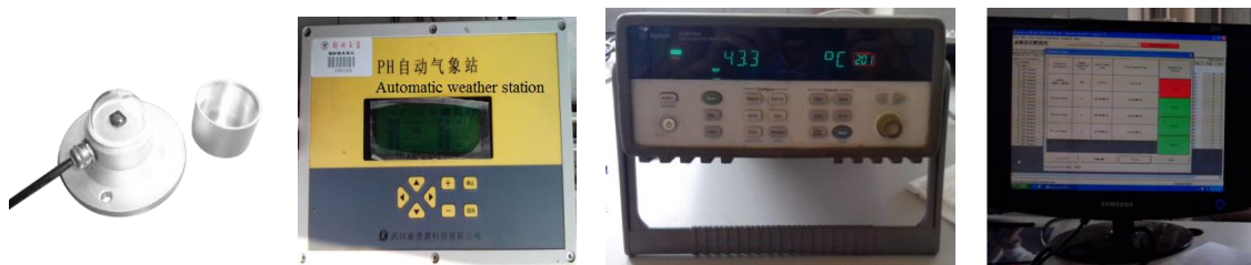
(a) Radiation sensor (b) Automatic weather station (c) Agilent data collection apparatus (d) Computer
