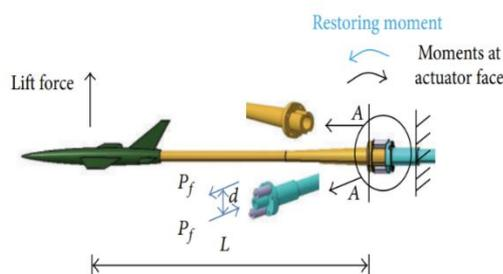
Figure 3 Sting-damping actuator design concept piezoelectric [10-17]
