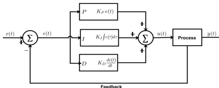
Figure 5 PID control block diagram, standard configuration of a PID control system [20]
