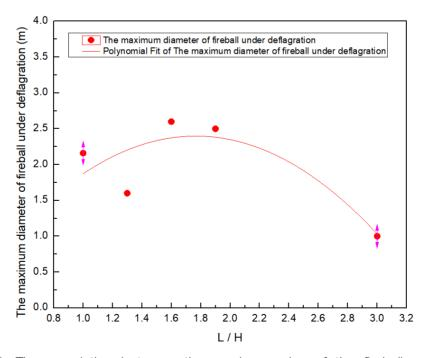
FIG.10. The correlation between the maximum size of the fireball and the parameter of the fragments, with the quality of 10g.
