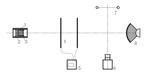
FIG.1 Experimental system; 1-Ballistic gun, 2-Sabot, 3-Fragment, 4-Velocity, measuring device, 5-Chronoscope, 6-High speed cinematography, 7-Surveyor's rod 8-Shield H6 explosive target.
