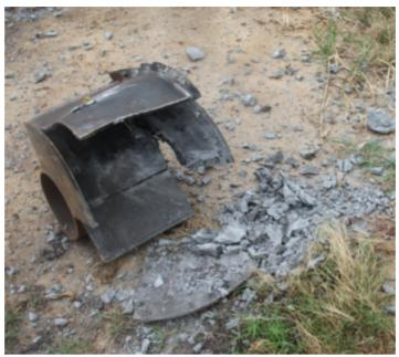
FIG. 3 deflagration of target (results of test for number 14)
