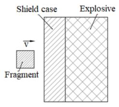
FIG.8. schematic diagram for the fragment impact on the shielded explosive
