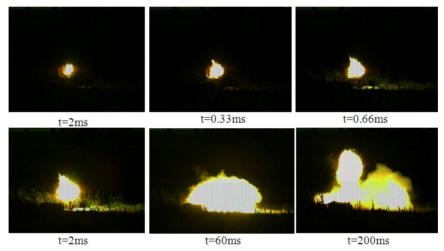
FIG.6 deflagration processes of target (results of test for number 14)
