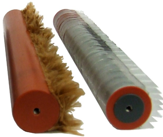
Figure 1: Photograph of the cylinders used in the present study left aft body fur right hairy flaps [5] hairy flaps for simulation
