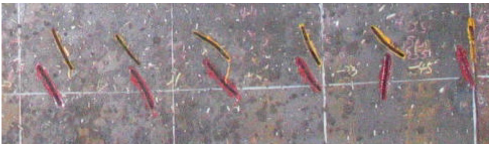
(b) Penetration of Target Plates at Distance of 5 Meters away from Warhead
