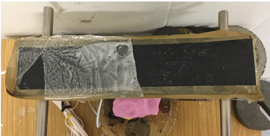
Figure 13: Failure in a 5 mm ice sample
